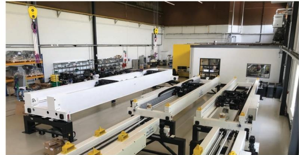
Ⓔ Cleanroom cranes being assembled by Mennens, using electronics from Elma.
