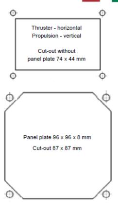
Panel plate is standard on motorized contollers. Vertikal dimensions motorized controller: 108 mm above and 92 mm below console panel.
